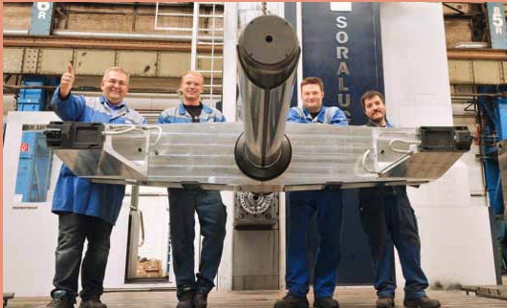
A new challenge for the SNT chippers: turning tool with 3,200 mm in diameter
