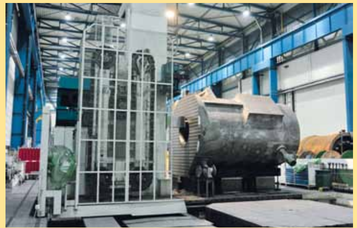
PAMA boring machine with part for Elektrostal's closed-die forging press
