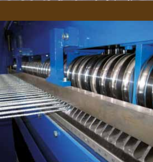
Outfeed area of cable tensing device with comb and guide roller
