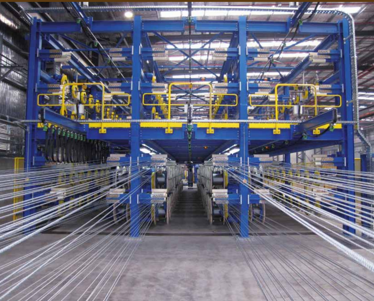
Two-story creel for 520 cables
