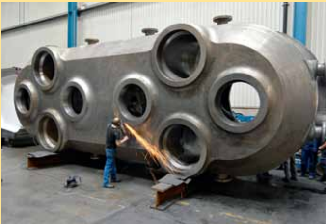
One of 14 parts for Alcoa's 50,000 t press
