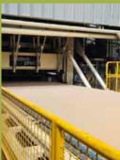
Infeed of the MDP mat into the Küsters press
