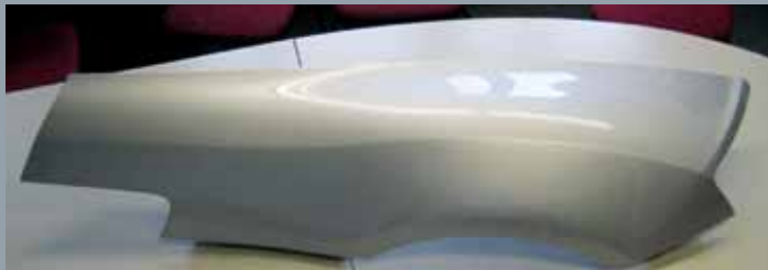
RTM fender for Audi
