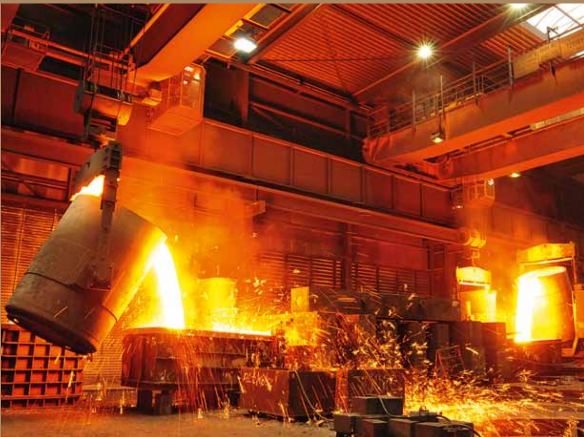
Casting: three pouring ladles of 150 t liquid iron forming a cross beam of 14 m length
