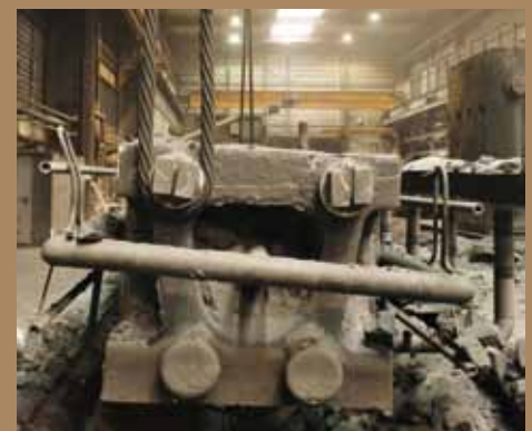
Drawing the casting from the molding pit
