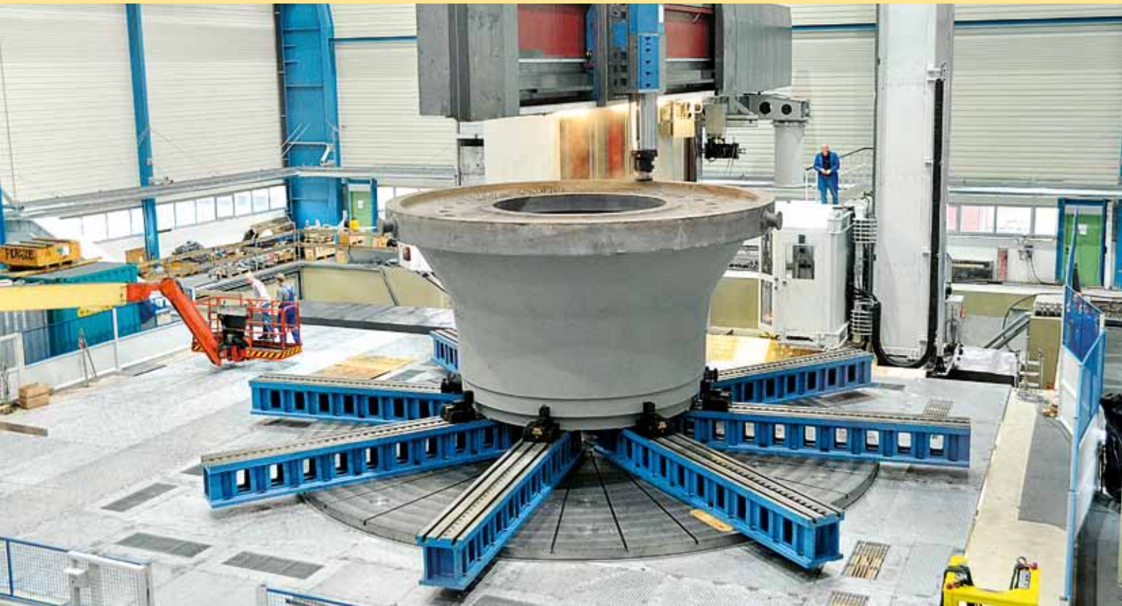
Vertical turning lathe type VME 10 by Schiess with grinding table
