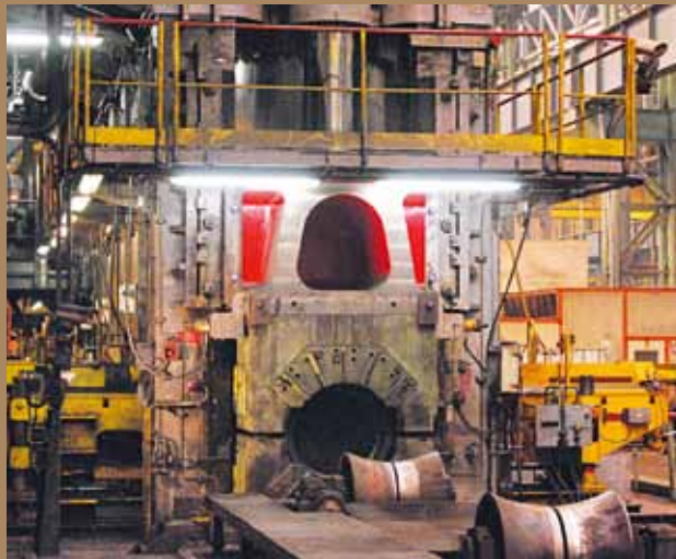
August 2011: The cross beam is installed and the pipe press is performing with the required level of power
