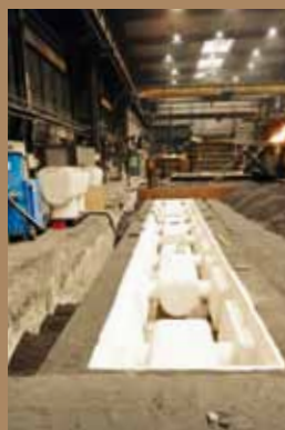
Cross beam during molding
