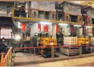
August 2011: The cross beam is installed and the pipe press is performing with the required level of power
