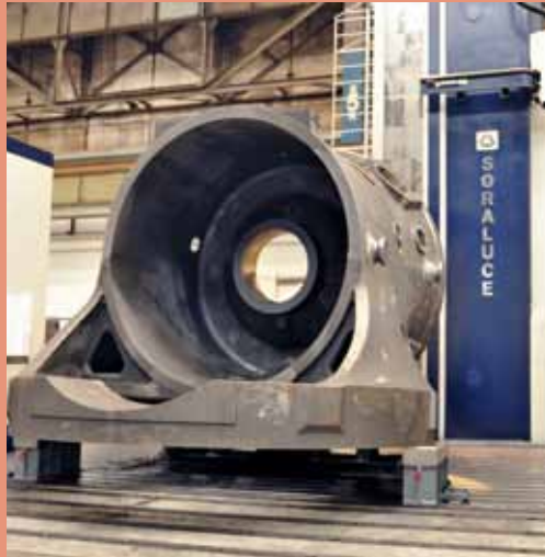
Machine carrier on the new traveling column drill
