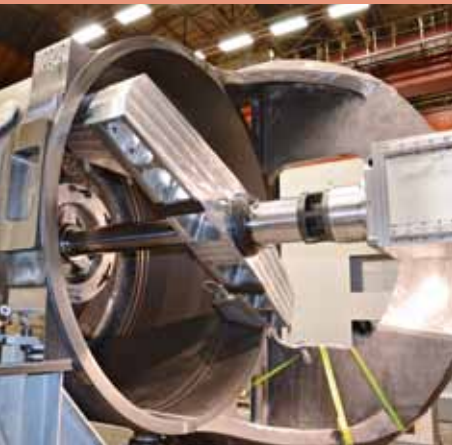
Highly demanding turning of the fit for an accurate assembly of the wind energy plant
