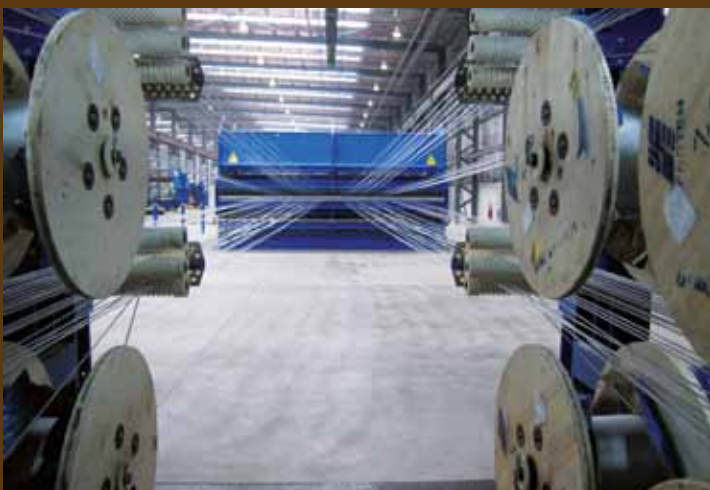
Infeed area of the cables into the tensiing device
