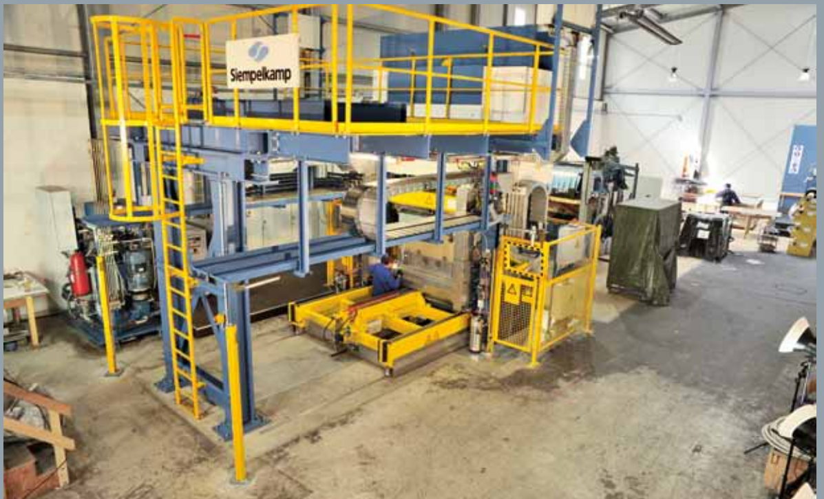
Special press for the production of RTM structures and Organosheet with loading unit
