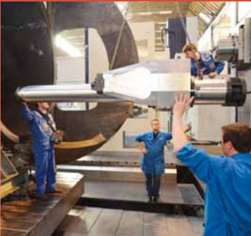
Positioning of the turning tool inside the machine carrier
