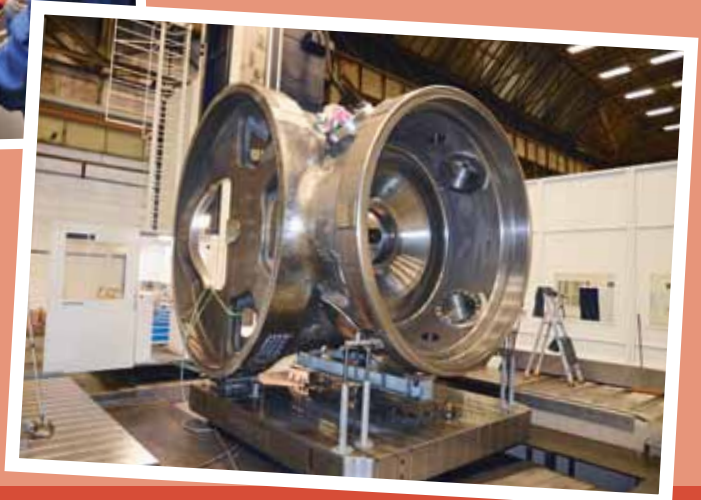
Ready to rotate in the air: machine housing equipped with lifting means
