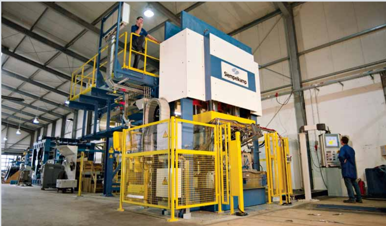
Special press for the production of RTM structures and Organosheet with loading unit
