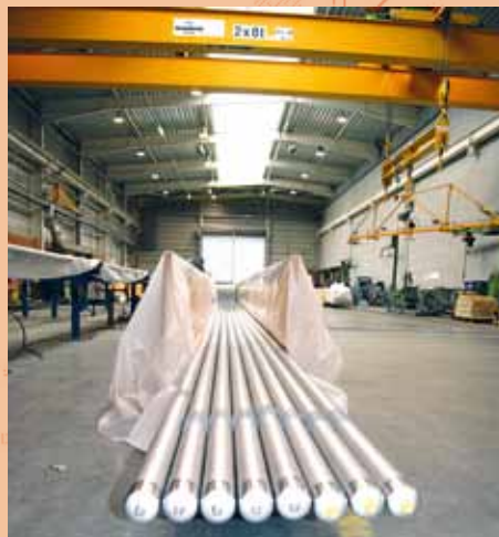
Transport of produced pipes with the Siempelkamp crane system
