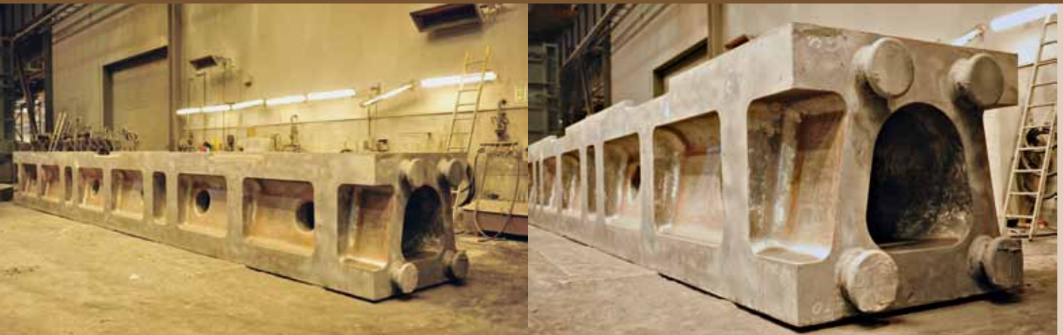
Press beam after the fettling shop
