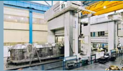
Component piece on the portal milling machine
