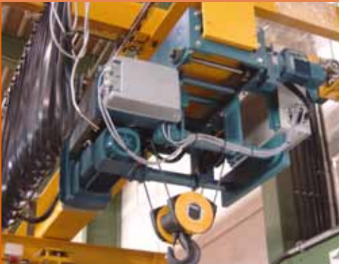
Special monorail trolley for latching crane
