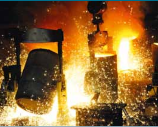
Pouring from four ladles simultaneously
