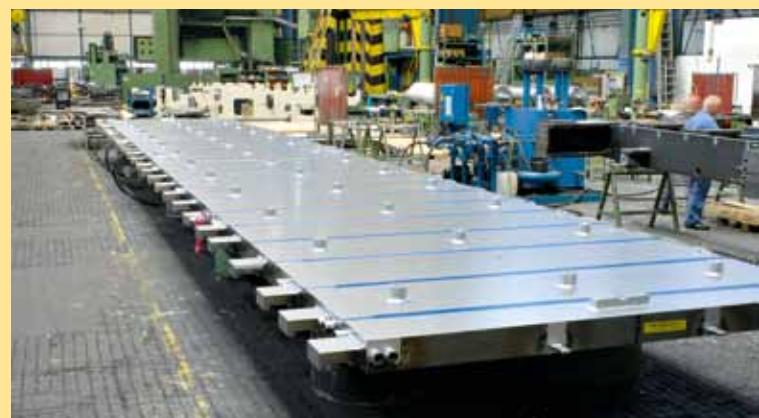
Machining of hot platens with a length of up to 18 m
