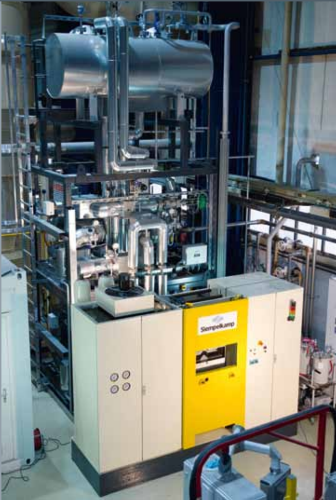
Laboratory press for the production and post-forming of Organosheet
