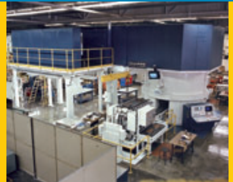
Rubber pad press for McDonnell Douglas
