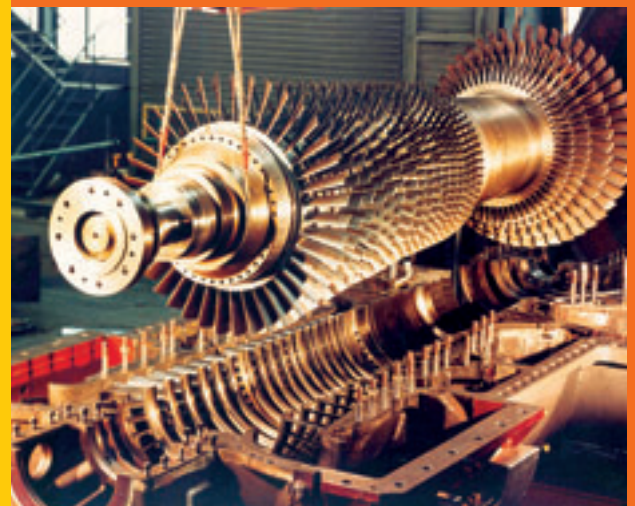
Mounting of a 168 megawatts gas turbine rotor (Photo: Siemens)
