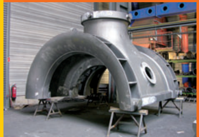
Raw casting of the upper shell of a steam turbine
