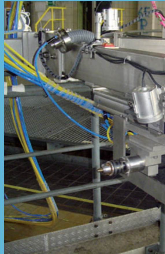
(Figure 3) Tool carrier with pneumatic drilling machines, dose rate measurement sensors and underwater video technology
