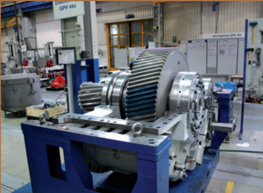
The gearboxes from Bosch Rexroth on a transport platform from STROTHMANN.
