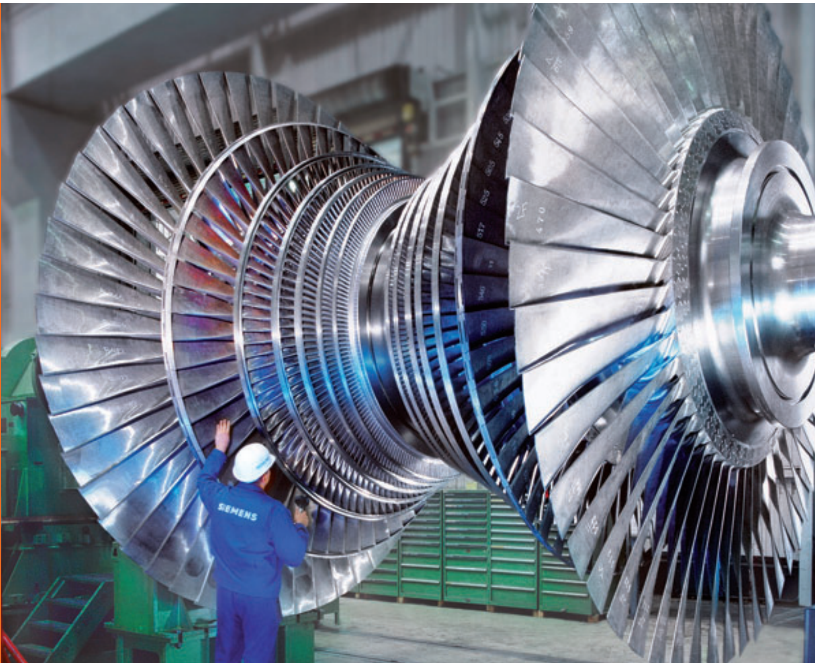
Steam turbine for Niederaussem (Photo: Siemens)
