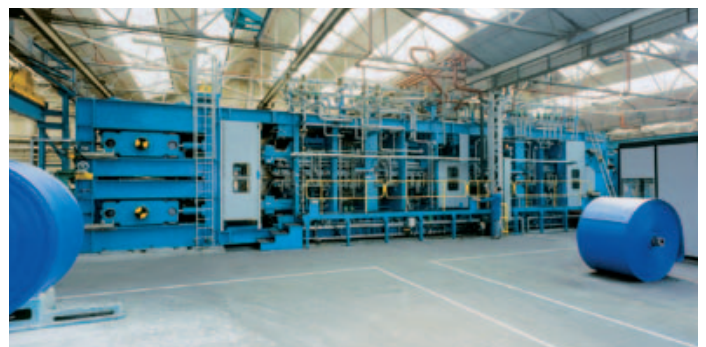
Siempelkamp double-belt press for PVC and rubber conveyor belts
