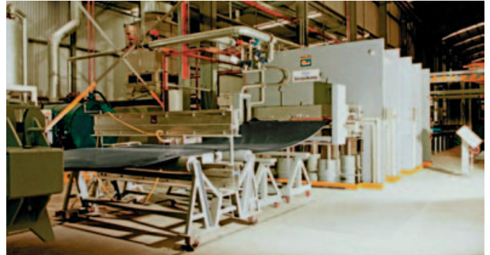
Conveyor belt repair press
