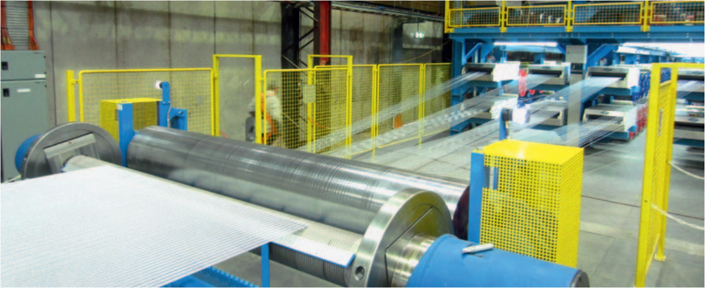
Direct tensioning system with roller comb
